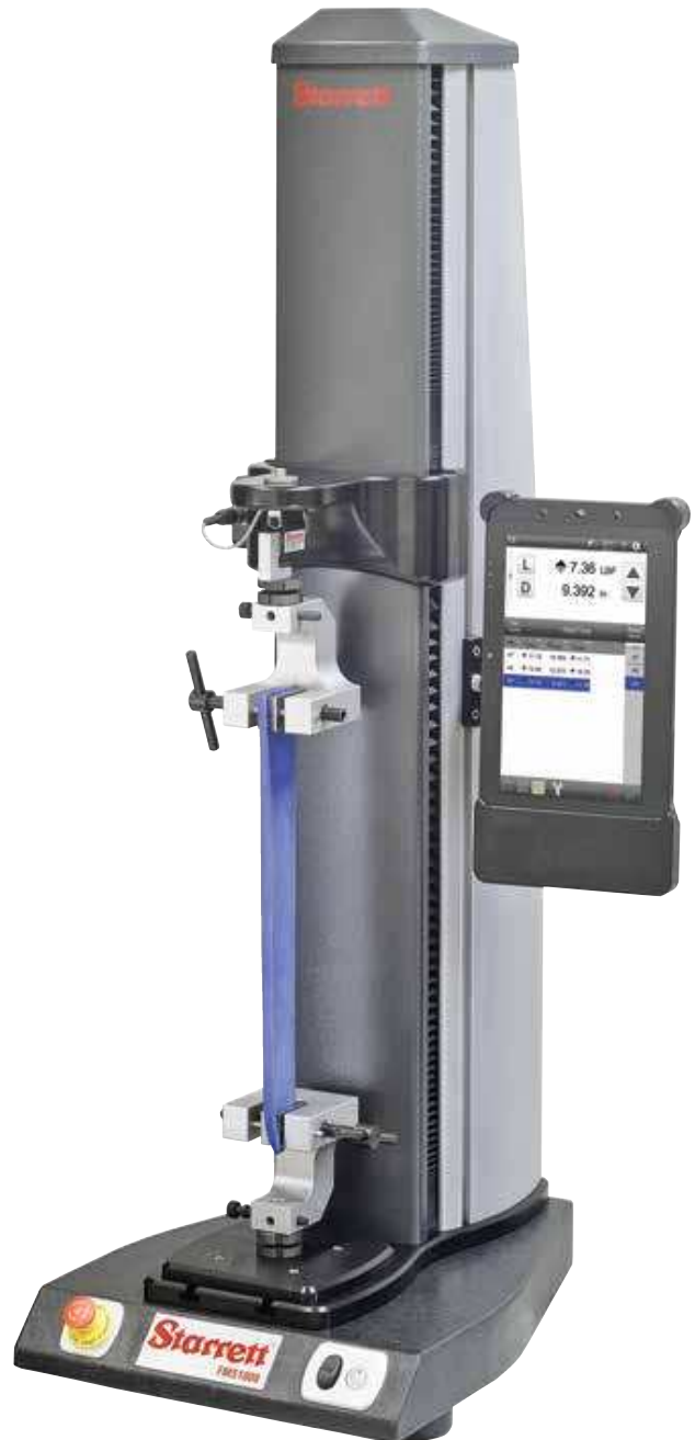
FMS-1000 Series with L2 Series software and tablet PC for force measurement applications
